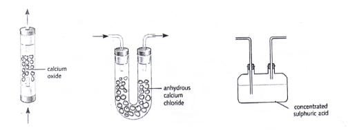
The first setup can ONLY be used for solid drying agents.
